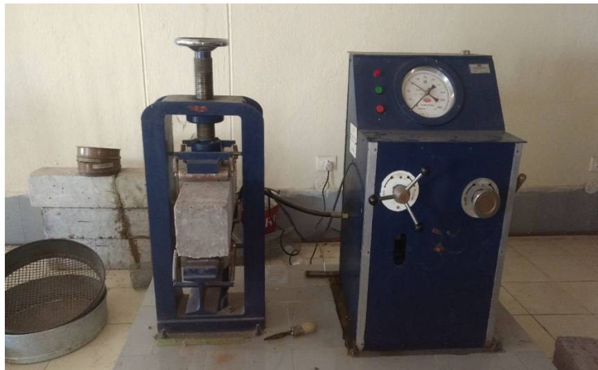
Fig.8. Loading specimen for flexural strength test on UTM
