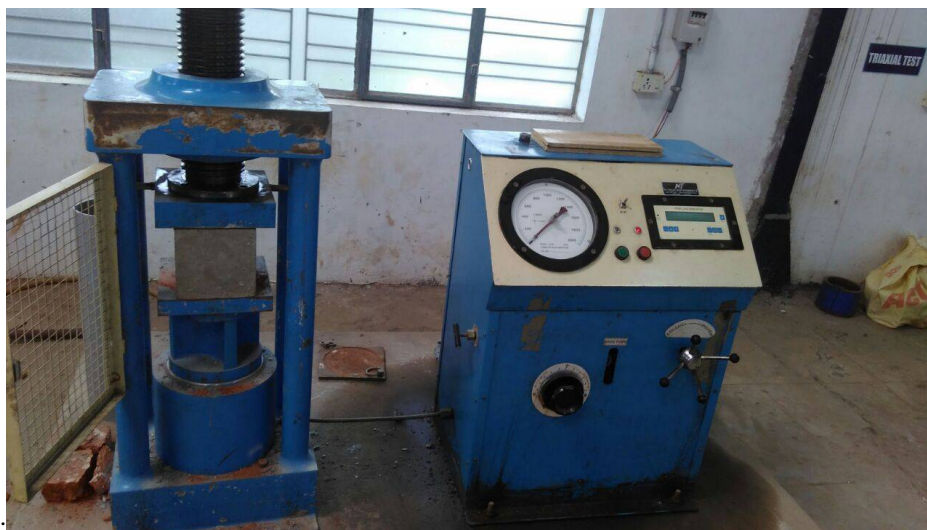
Fig.7. Loading test specimen for compressive strength test on UTM
